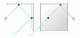
**Transmissive Dihedral Corner Reflector Array** As its name suggests, this reflector consists of two orthogonal specular surfaces that reflect the light to project images. The first angle of incidence and the second angle of emergence both have the same reflection angle, and the plate acts as a projection surface for displaying images in mid-air at a 1:1 ratio.
