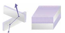
The Essential "Made in Japan" Technology The plate consists of methodically-positioned vertical mirrors mere hundreds of microns in size. While the plate may seem like a simple two-layered mirror structure at first, the mirror positioning can only be achieved with the cutting-edge manufacturing technology typical of products "Made in Japan".
